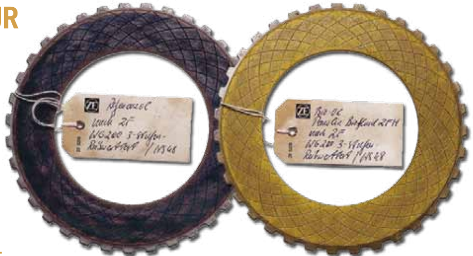
Lamella comparison according to WG 200 3-stage friction coefficient test (left: reference oil; right: PANOLIN BIOFLUID ZFH)
